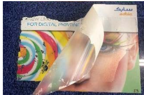
DELAMINATION ON UNCOATED FILM
